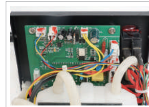
All in 1 PCB Metal screws fixed.
