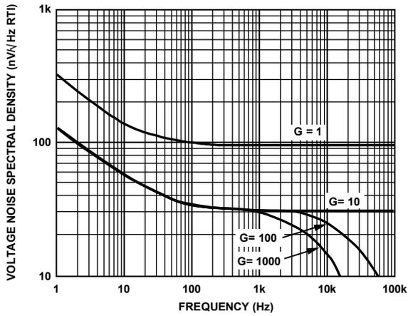
Figure 10. Voltage Noise Spectral Density vs. Frequency
