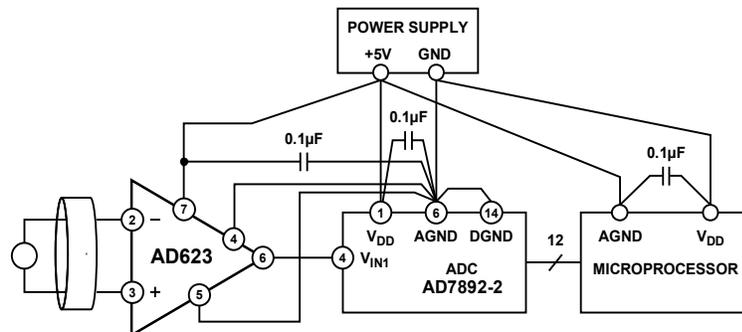
Figure 48. Optimal Ground Practice in a Single-Supply Environment
