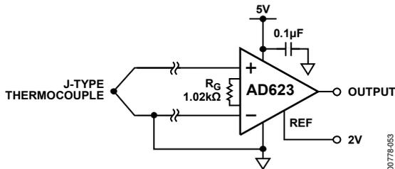
Figure 54. Amplifying Bipolar Signals with Low Common-Mode Voltage
