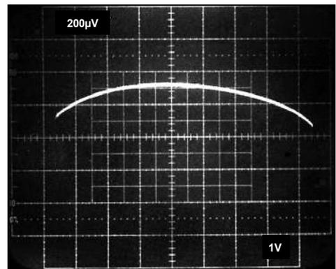
Figure 37. Gain Nonlinearity,  $G = -1$  (50 ppm/DIV)
