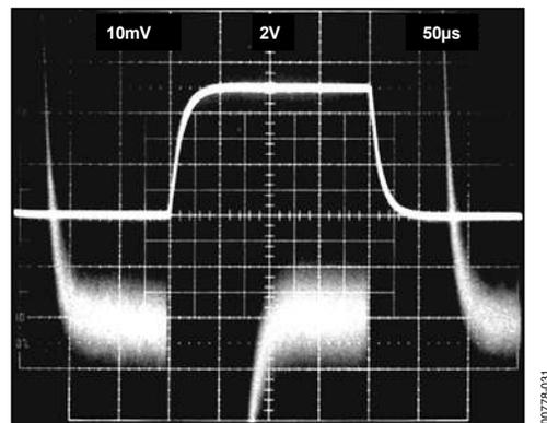
Figure 31. Large Signal Pulse Response and Settling Time,  $G = 100$ ,  $C_L = 100 pF$
