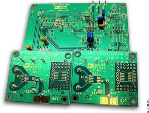
Figure 56. Evaluation Boards for Analog Devices In-Amps
