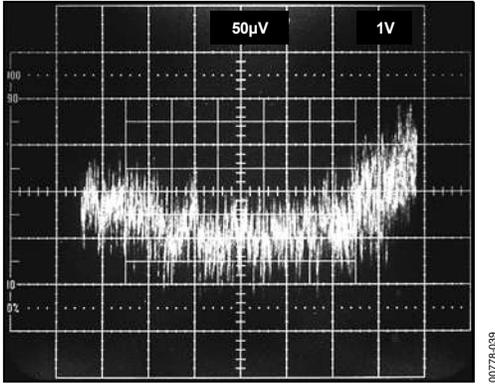
Figure 39. Gain Nonlinearity,  $G = -100$ , 15 ppm/DIV
