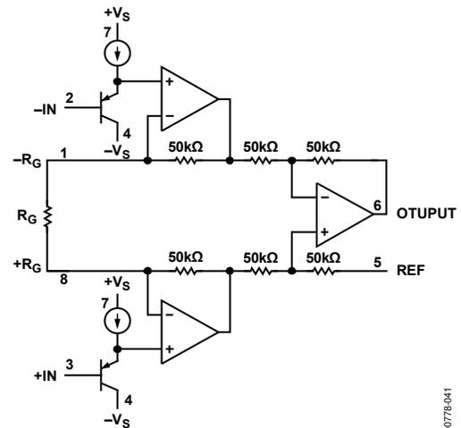
Figure 41. Simplified Schematic
