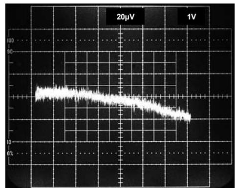
Figure 38. Gain Nonlinearity,  $G = -10$  (6 ppm/DIV)
