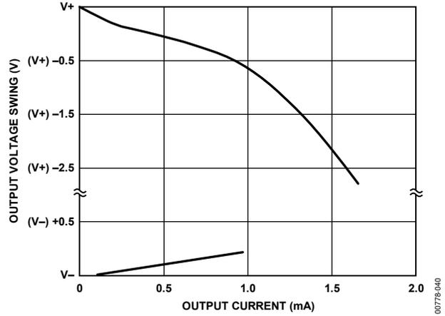
Figure 40. Output Voltage Swing vs. Output Current
