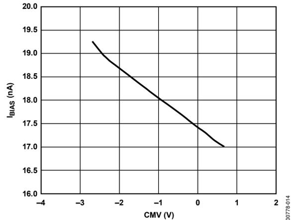
Figure 14. I<sub>BIAS</sub> vs. CMV, V<sub>S</sub> = ±2.5 V
