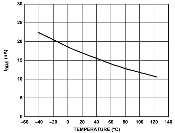
Figure 12. I<sub>BIAS</sub> vs. Temperature
