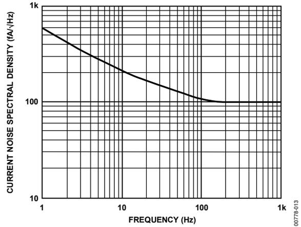
Figure 13. Current Noise Spectral Density vs. Frequency
