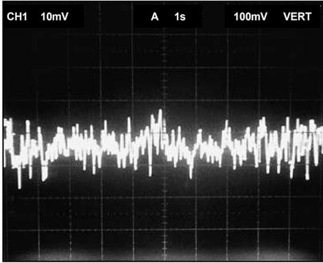
Figure 15. 0.1 Hz to 10 Hz Current Noise (0.71 pA/DIV)
