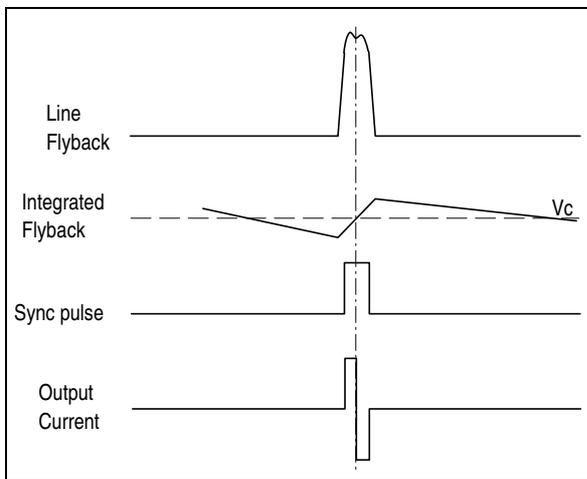
The sync-pulse drives the current in the comparator. The line flyback integrated by the external network gives on pin 13 a saw tooth, the DC offset of this saw tooth is fixed by VC. The comparator output provides a positive current for the part of the signal on pin 13 greater than VC and a negative current for the other part. When the line flyback and the video signal are synchronized, the output of the
