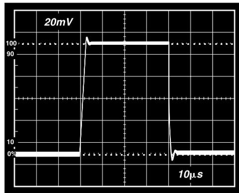
Figure 24. Small Signal Response,  $G = 10$ ,  $R_L = 2 \text{ k}\Omega$ ,  $C_L = 100 \text{ pF}$
