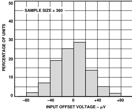
Figure 3. Typical Distribution of Input Offset Voltage
