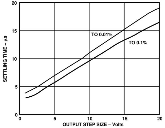
Figure 29. Settling Time vs. Step Size ( $G = 1$ )
