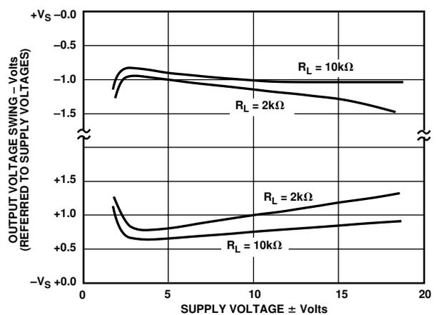
Figure 19. Output Voltage Swing vs. Supply Voltage,  $G = 10$
