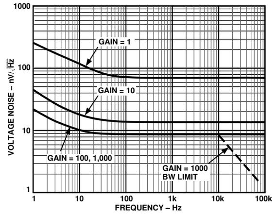
Figure 8. Voltage Noise Spectral Density vs. Frequency, ( $G = 1-1000$ )
