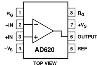
1000. Furthermore, the AD620 features 8-lead SOIC and DIP packaging that is smaller than discrete designs, and offers lower power (only 1.3 mA max supply current), making it a good fit for battery powered, portable (or remote) applications.
