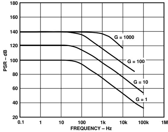
Figure 14. Positive PSR vs. Frequency, RTI ( $G = 1-1000$ )
