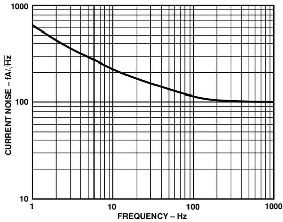
Figure 9. Current Noise Spectral Density vs. Frequency
