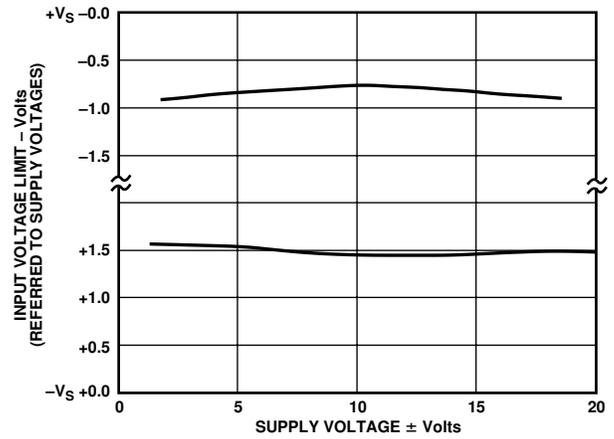
Figure 18. Input Voltage Range vs. Supply Voltage,  $G = 1$
