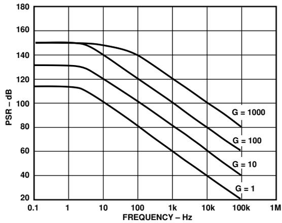
Figure 15. Negative PSR vs. Frequency, RTI ( $G = 1-1000$ )
