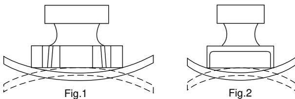
The arrangement shown in Fig.2 is more effective in preventing stress than that shown in Fig.1.
